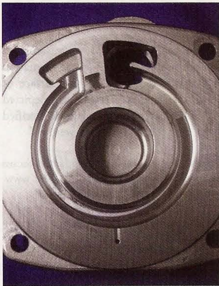
Above is an optimized hydraulic cavity.
