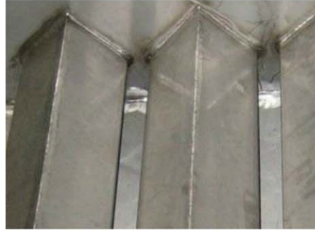
From left to right: If space is a premium, Coagulants and flocc agents can be added within the piping manifold. Note the sampling ports added in this one. Next, a sloped bottom design makes removing settling solids much easier. The photo on the right shows a liquid solids separation system designed and built by P.E.W.E.
